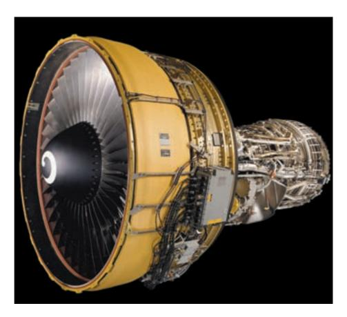
levels. CF6-80 maintenance shop visits will be few and far between as gas path deterioration is commendably low when the engine is utilised on long-haul operations.
